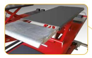
·Lift table with double lifting cylinder and double extensions, in front and rear, which is very flexible, no movement of vehicle on the lift needed.
