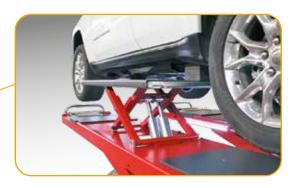
•Lift table with double lifting cylinder to ensure a constant parallel lift movement.
